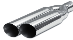
(Staggered) SS253518 3.5" Dual Outlets, 2.5" Inlet, 18.0" OA Length, Angle Cut, Clamp-On or Weld-On
