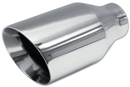
SS254590 4.5" Outlet, 2.5" Inlet, 9.0" OA Length, Double Wall, Angle Cut, Clamp-On or Weld-On
