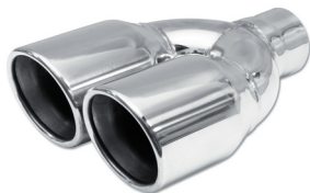
(Non-Staggered) SS22535975 3.5" Dual Outlets, 2.25" Inlet, 9.5" OA Length, Double Wall, Rolled Edge, Angle Cut, Clamp-On or Weld-On
